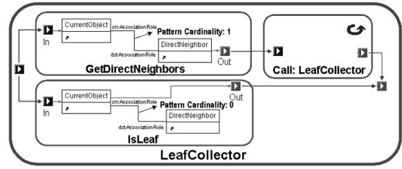
Fig. 7. Structure of Leaf Collector Pattern [37]
