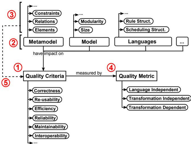
Fig. 5. Quality Framework for MDE (adapted to Model Transformation)
