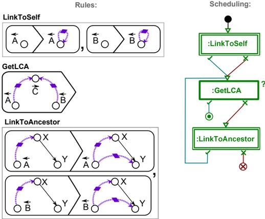
Fig. 12. The second set of rules to solve LCA problem.
